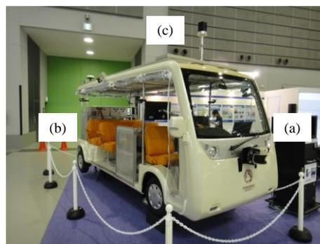
Fig. 2 (a) manufactured large EV, (b) in-wheel motor controller, (c) omnidirectional cameras. Coil for wireless charging is installed under the car.
